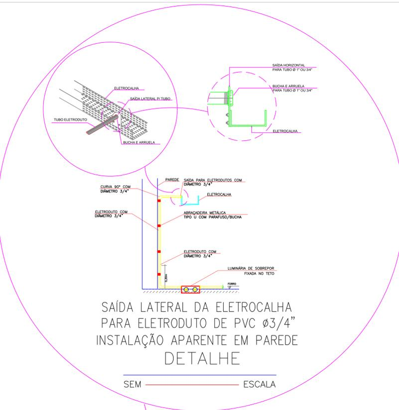
SAÍDA LATERAL DA ELETROCALHA PARA ELETRODUTO DE PVC Ø 3/4\"/>
